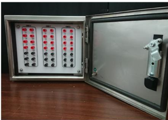
Five-way binding post terminals for simple banana plug connections
