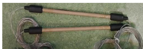
MMO coated titanium auxiliary electrode (or cathode)
