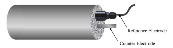
LPR Corrosion Monitoring System is to monitor the rebar corrosion condition of existing concrete structures. By installing precast LPR Probe in a core hole, the variations of the corrosion rate surrounding the LPR probe can be measured. LPR Monitoring System is useful to determine:
