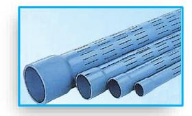
Slotted PVC gas vent pipe is a specialty product that can be used in cathodic protection deep anode wells to displace chlorine gas generated by the discharge of DC current from the impressed current anodes.
