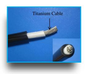
Corrosion free titanium cable is used to prevent the cable failures caused by corrosion. Even though the cable insulation is physically damaged during the anode installation or deteriorates due to the limited life, the titanium cable can maintain to carry current to the anodes.
