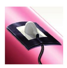
Handy Cap XL IP is a prefabricated assembly designed to provide quick, field-applied corrosion protection to anode and test lead wire welds on metal pipe and tanks. This economical product is ideal for use in limited access applications. New Handy Cap XL IP now adds the innovative technology of Tapecoat Gray Adhesive to its unique design. The integration of a primer in Tapecoat Gray makes field application of Handy Cap XL IP easier and more economical.
