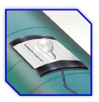
Handy Cap IP is a prefabricated assembly designed to provide quick, field-applied corrosion protection to anode and test lead wire welds on metal pipe and tanks. This economical product is ideal for use in limited access applications. Handy Cap IP adds the innovative technology of Tapecoat Gray Adhesive to its unique design. The integration of a primer in Tapecoat Gray makes field application of Handy Cap IP easier and more economical.
