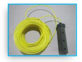
**ProCell Zinc Reference Electrode** is designed to use in seawater. It consists of high purity metallic zinc rod. The reference potential of a zinc element in seawater is about 1.1 volts negative to that of a saturated  $Cu/CuSO_4$  reference electrode.
