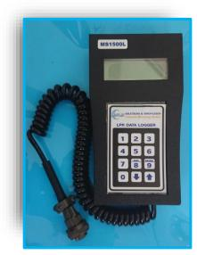
MS1500 LPR meter is a hand-held, 9 volts battery-powered, intrinsically safe corrosion meter capable of measuring and storing data from linear polarization resistance (LPR) corrosion rate probes. The instrument is light weight, microprocessor-based, and features a simple, menu-driven interface using a 12-key keypad and a 4-line LCD display.
