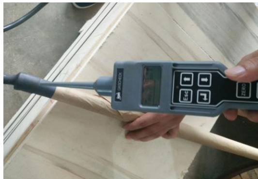
Helium leak test
