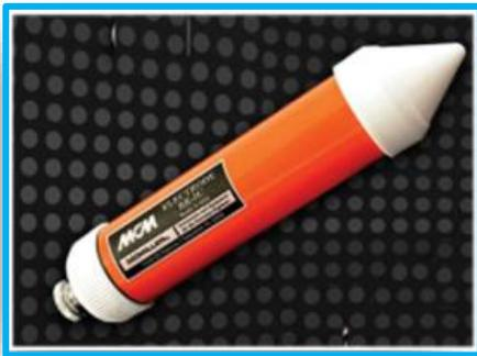
Copper/copper sulfate reference electrode with the rugged ceramic plug having a conical-shaped surface. Designed for use in soft soils. High purity copper rod and robust Lexan tube. The electrode has a transparent "window" to view the condition of the saturated copper sulfate solution. The saturated copper sulfate solution is prepared (inside the Lexan tube) by the end-user, according to the provided instructions. Supplied with a charge of copper sulfate crystals inside the Lexan tube.
