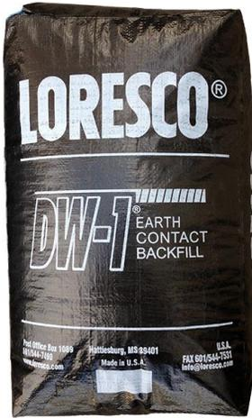
Loresco DW-1 Backfill is a sized carbon backfill with particles ranging between 0.1 to 1 mm. DW-1 weighs 74 lbs per cubic foot and sinks readily in water or light mud. The fixed carbon content of DW-1 is over 99%.
