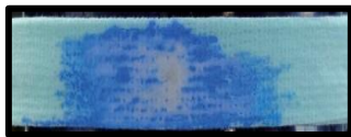
Ammonia Liquid or Gas (NH 3 , HH 4 ) 1% to 28%, pH 14.0 Light Blue → Navy Blue
