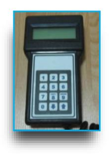
MUI-MS1500E meter is a hand-held, battery-powered, corrosion meter capable of measuring and storing data from all types of electrical resistance (ER) corrosion probes. The instrument is lightweight, microprocessor-based, and features a simple, menu-driven interface using a 12-key keypad and a 4-line LCD display.
