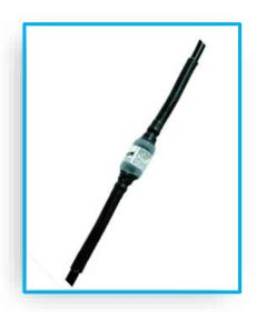
Ex isolating spark gaps EXFS KU are used for conductive system parts which cannot be interconnected directly in hazardous zones. This includes, for example, pipe sections supplied with a cathodic corrosion protection system.
