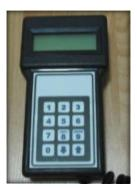
MUI-MS1500E meter is required for measurement. Handheld, battery-powered MS1500E is capable of measuring and storing data from ER corrosion probes.
