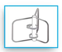
Centralizer is used in a groundbed hole to uniform CP maintain a more current distribution from the anode by ensuring backfill consistent cover. In addition, maintaining proper spacing between the anode and non-conductive gas vent pipe is an important function for the anode centralizer.
