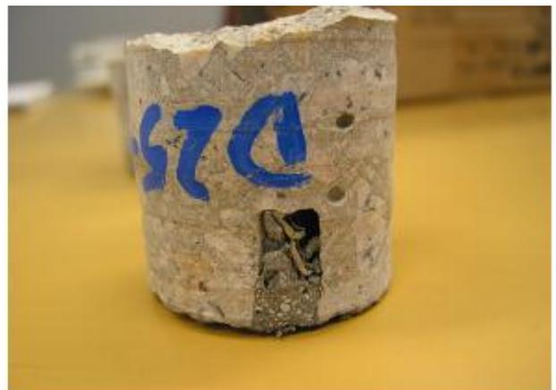
Figure 10. Poor grouting condition in slot
