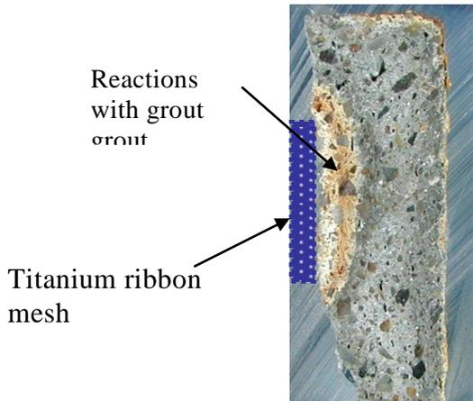
Figure 5. Discoloration of the grout surrounding The ribbon mesh in the slot
