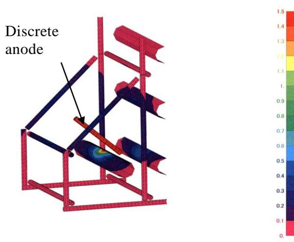
Figure 3. Current distribution from the discrete anode in the beam.
