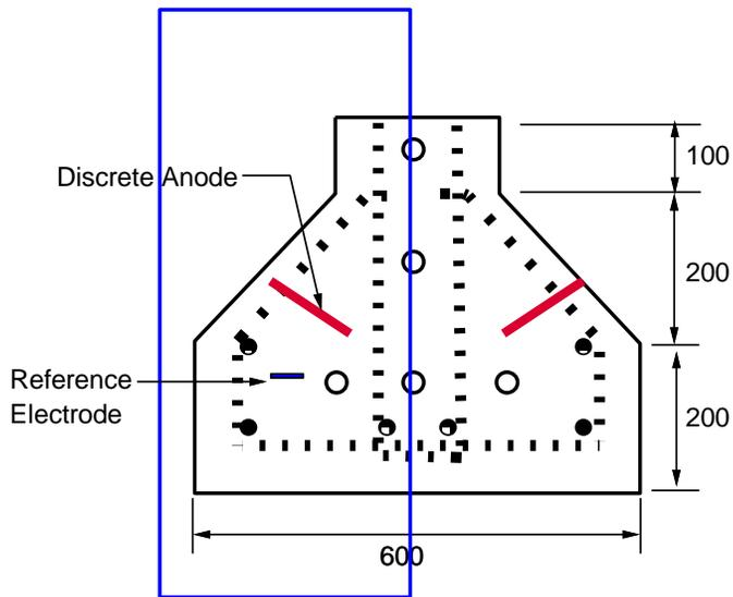
Figure 1. Configuration of discrete anode position in prestressed concrete beam
