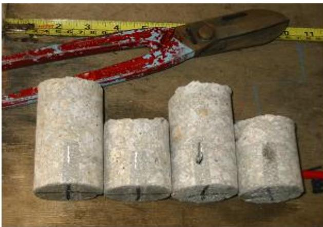
Figure 9. Grouting conditions inspecting by cores
